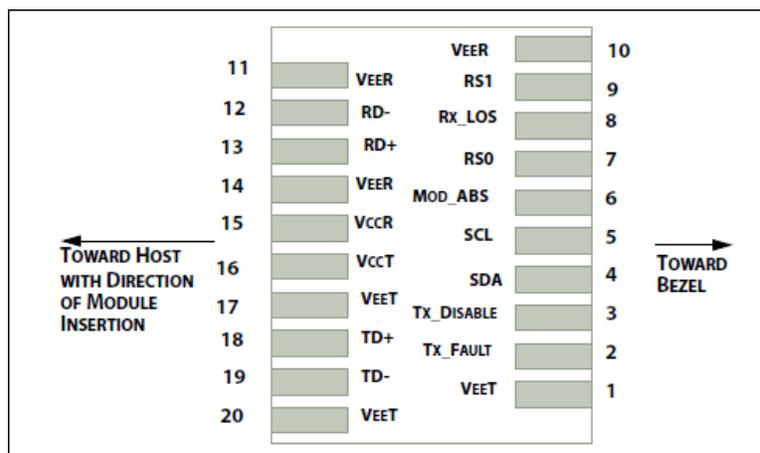
Figure 7: SFP56 Module Pin Map
